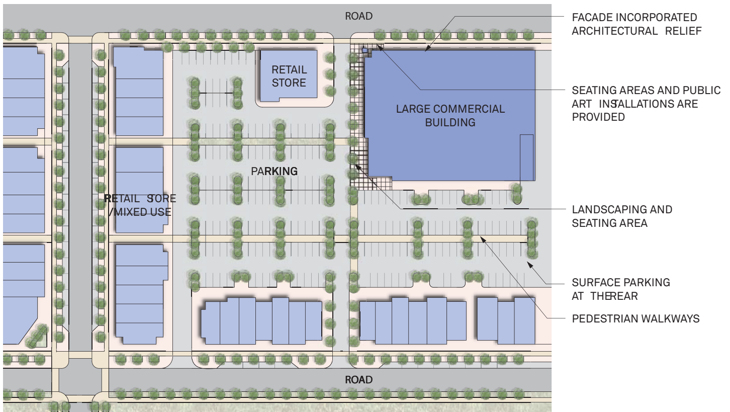
Illustration demonstrating a potential layout for a large-format retail development, with the building at the property line and parking located internally to the site (or screen where adjacent to the sidewalk).
