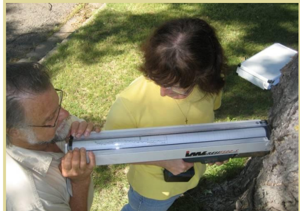
The City Forester assists with the use of a resistograph to determine the presence of internal decay on a street tree.
