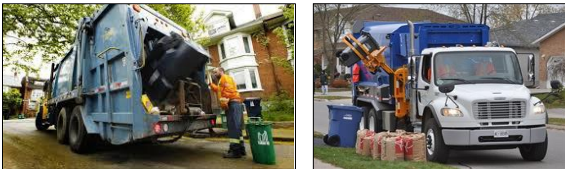
Figure 5: Lift Assist (left) and Automated Collection (right) 5
