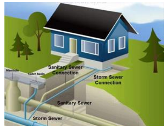
Sewer Connection from the home to the sewer main
